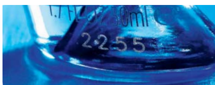
7031 Scribing laser High quality mode (stroke fonts)
